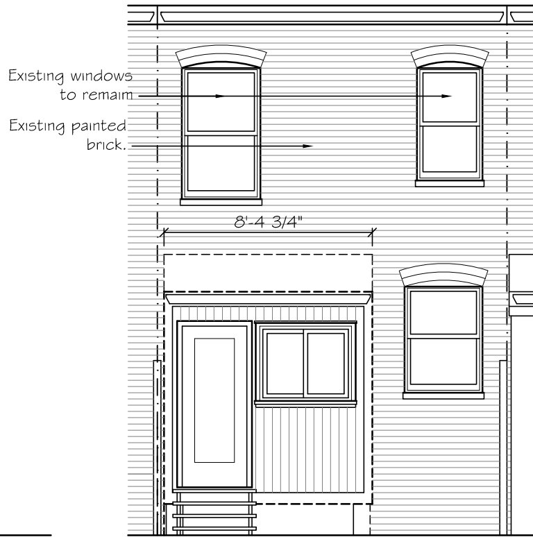
2 Existing Southeast Elevation A-4 3/16" = 1'-0"
